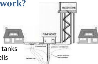
are automatically turned on. The wells pump water into our distribution pipes and to the water tanks. Once the water tanks are full, the wells shut down. This process takes about 8 to 12 hours depending on the actual use during the filling process. Many residents have wells located near their homes, but for the most part, everyone receives a blended mix of water from each of the wells.
